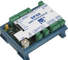
The user of SPA8 can select each of two analog inputs as voltage (0 to 10V), current (0 to 20mA) temperature (for cheap sensors KTY81-210 and precise Ni5000 temperature sensors) or for function like another logical input. The analog values measured on inputs can be send in SMS in actual user units and values like 7.9 MPa or 735 kg (configurable recalculation including non linear functions included).
