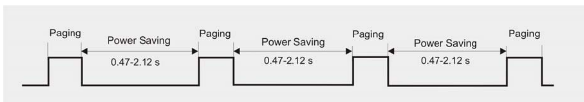
Figure 43: Power saving and paging in GSM networks
