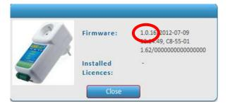
I want to find out what version of station FW I have. I connect the station via USB cable. Click on the **Monitoring** tab, then in this tab click on the **More** ... Current version of station FW is 1.0.16.
