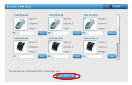
At the bottom of the window, click on the *Load from File*. Select a file with a saved configuration and then click on the *Open* button. Wait for a while. This will load the configuration from a file.
