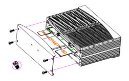
9. Installing DIN-rail Kit (2 screws)
