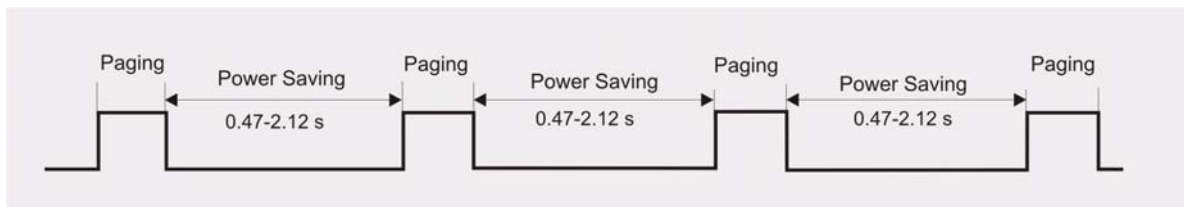
Figure 8: Power saving and paging in GSM networks
