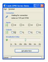
*Details:* Program listens on TCP port 5700 for incoming connection. Port 5700 is default port where CMGSM connects to. Program periodically queries status of inputs X0-X3 from remote station. You can change any of output Y0-Y3 by click on a check box Y0-Y1.
