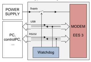
Time, which is still not considered an error of modem is configured using commands via serial interface RS232. USB port is not possible to use for Watchdog setting!
