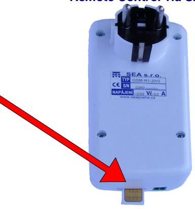
Device status – Send an SMS in form 1234 STATE to a phone number of the SIM card which is inserted into the GSM R1 ZAS. The device will send back an SMS with current device status. E.g.: GSM R1 ZAS: ON, Signal= 54%, Temp=28°.
