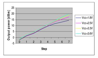
Figure 2: Typical Transmitter RF power out
