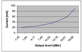
Figure 1: Typical module supply current in TX mode (with firmware test)
