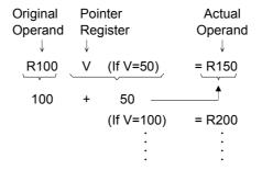
As shown in the above diagram, you only need to change the V value to change the operand address. After combining the index addressing with the FBs-PLC function instructions, a powerful and highly efficient control application can be achieved by using very simple instructions. Using the program shown in the diagram below as an example, you only need to use a block move instruction (BT M) to achieve a dynamic block data display, such as a parking management system.
