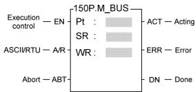
Pt : 1~4 , specify the communication port to work as the Modbus RTU master
